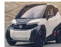
This is an **electric two-seater** with an **autonomy of 125 km**, a maximum speed of 45 km/h, 2.28 m in length by 1.29 m in width, and a removable battery. **Through the "My Silence" app**, it is possible to enter the vehicle, start or stop it, activate the air conditioning, lock the doors, etc.
