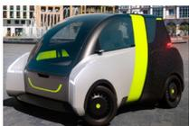
This is **driven with a joystick** located between the 2 front seats and has **cameras instead of side mirrors** to show the driving image on the screen. Its length can be expanded by 37 cm to seat 4 people. Its **2 and a half metres** in length mean it can be parked perpendicularly.
